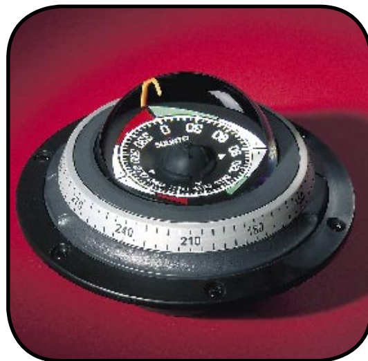
K-95 is supplied with flush mounting that screws into the deck. This makes it easy to detach the compass for transport. When detached, the mount hole is covered with a hatch. K-95 is also available with mast/bulkhead and surface mounting.
